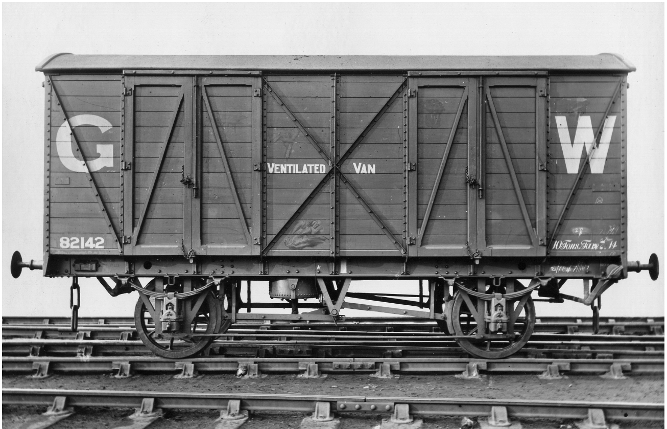
Mink C No. 82142 with 25 inch "G" and "W" painted across the diagonal strapping. This image appears in "Great Western Way" but this version should be clearer. GWR
